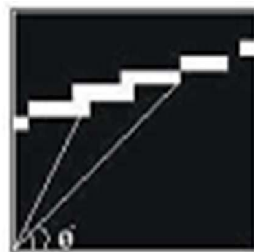
Fig. 6: Finding the angle of each white pixel and calculate the mean value
